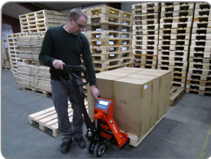
WSP 2200 transports and weighs goods in the same work process.
