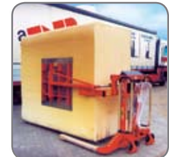
Straddle Logiflex with special gripping arms for foam blocks.
