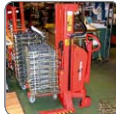
Logiflex with very short forks being used for the handling of wire frames.
