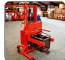
Logiflex with side-tilting forks and spear to carry and turn wire box.
