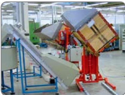
Logiflex with side-tilting forks being used when lifting and emptying components on a production line.
