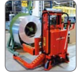
Logiflex with fixed drum fork carriage for the carrying of heavy reels with large diameters.
