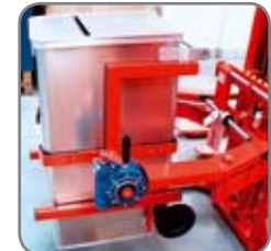
Logiflex revolving a dustbin (drum turner principle).
