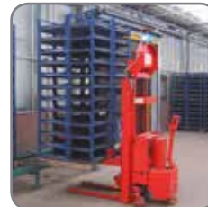
Fully powered Logiflex, remotely controlled from central computer, being used to deliver empty pallets to a production line.
