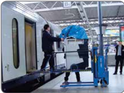
Logiflex with ramp, being used to carry trolleys in and out of trains.
